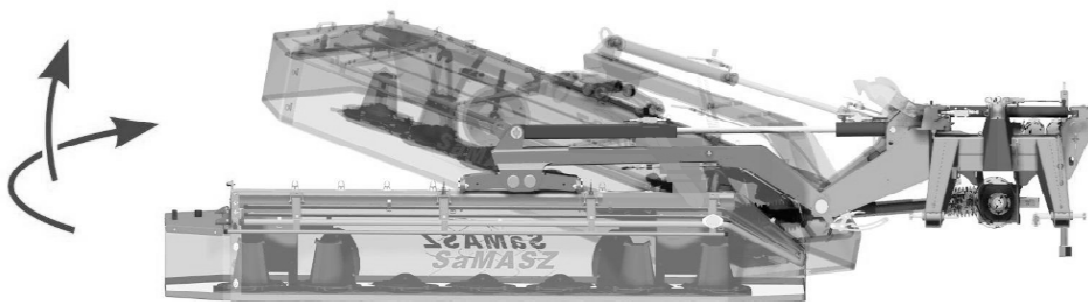
Fig. 10. Simultaneous holding back of the mower up and backwards when safety breakaway advice is used
