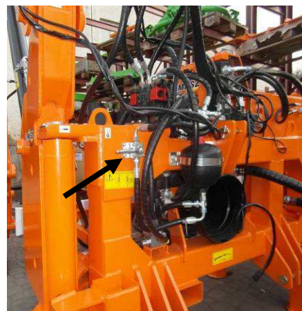
Fig. 68. Pressure reduction valve in unloading system
