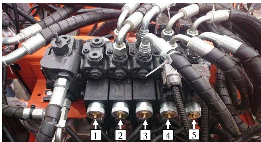
Fig. 64. Hydraulic distributor EP – description of distributor functions Camel 900 EP, KWT 650 EP, KWT 651 EP: 1 - turntable, 2- arm extension, 3- 2nd extension arm, 4- main extension arm, 5- cutting part; KWT 550 EP: 1- turntable, 3- 2nd extension arm, 4- main extension arm, 5- cutting part
