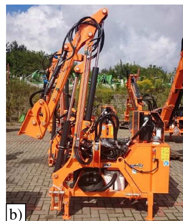
Fig. 67. Correct machine storage position: a) KWT, Camel, b) KOLIBER
