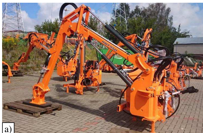
Fig. 67. Correct machine storage position: a) KWT, Camel, b) KOLIBER
