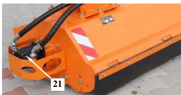
Fig. 62. Hydraulic engine driving shaft with cutterbar's knives
