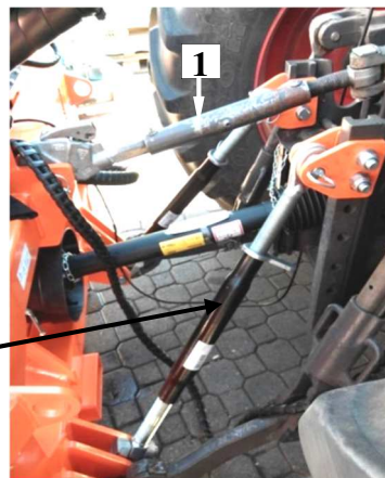
Fig. 27. Machine mounted on tractor's rear 3-point linkage
