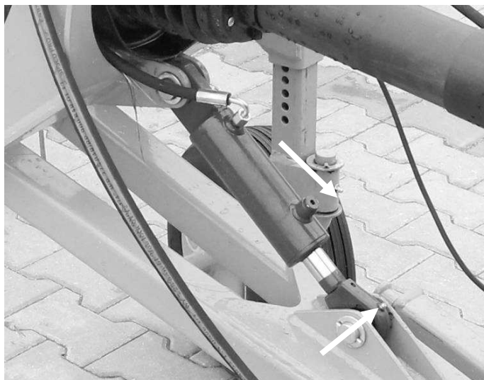
Fig. 41. Lubrication points on joints
