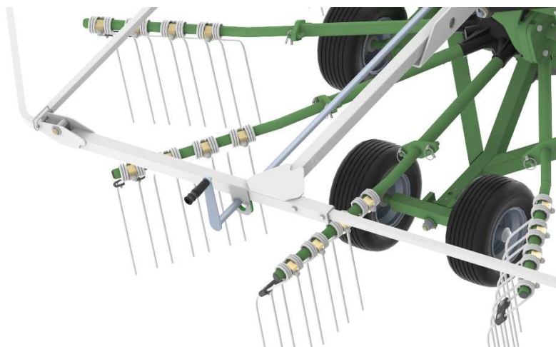
Fig. 15. Working height adjustment lever
