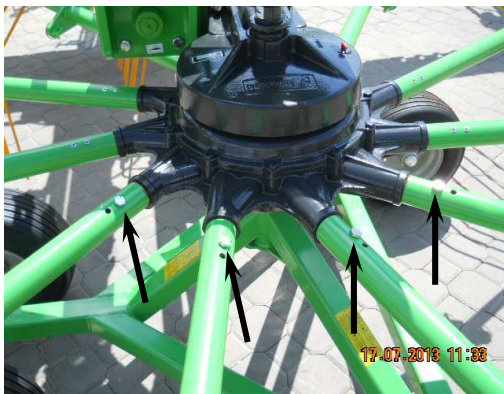
Fig. 10. Provisional mounting of rake arms with bolts
