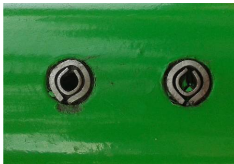
Fig. 13. Properly hammered pins
