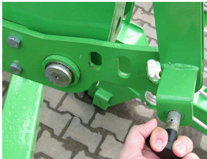
Fig. 20. Working width adjustment possible
