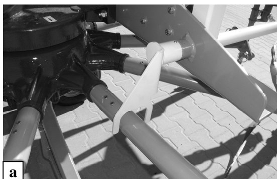
Fig. 13. a) Locking the gear for transport (guard lifted vertically), b) Locking the gear for operation (guard lowered horizontally)
