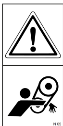
N-05 CAUTION – belt transmission, be extremely careful!
