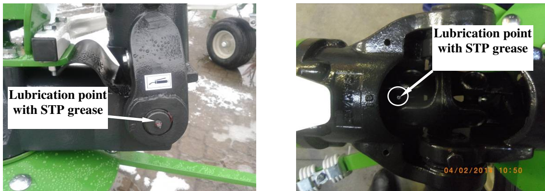
Fig. 26. Lubrication points of the joints
