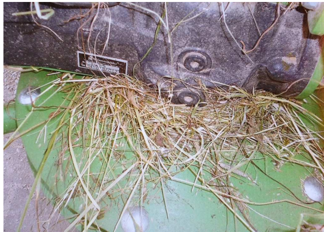
Fig. 22. Wrapped grass under the gearbox
